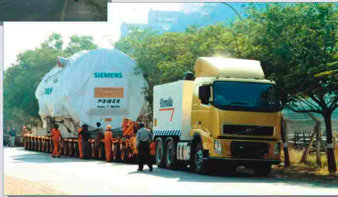
Turbine having dimension 10.93m x 5.20m x 4.86m - 310 MT loaded on 20 nos Goldhofer hydraulic axles trailer.
