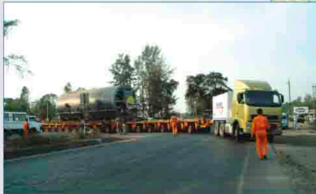
Generator 12.51m x 4.5m x 4.5m – 340 MT loaded on 20 nos Goldhofer hydraulic axles trailer.
